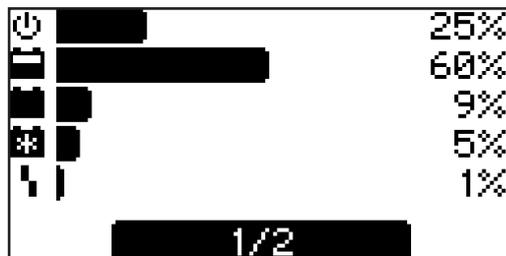
In statistics mode, horizontal bars display the frequency of the following device operating statuses:
