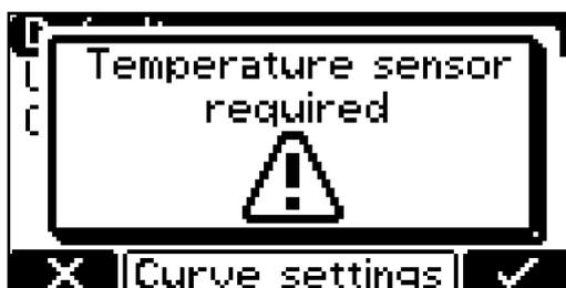
A note is displayed if a characteristic that requires an external temperature sensor is selected.
