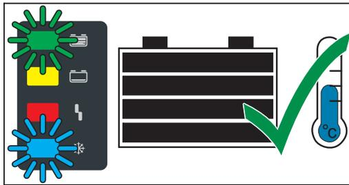
For an optimal battery life, only disconnect the battery from the charger when the blue "Battery cooled" indicator is showing in addition to the green indicator, in accordance with the explanation below. If several chargers are in use, first disconnect the battery which has been fully charged for the longest (the coolest).
