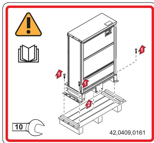
Remove the device from the pallet after delivery.
