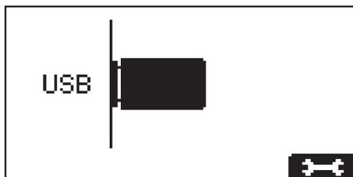
In USB mode, the display shows whether or not a USB flash drive is connected.
