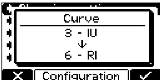
If the setting is not confirmed, the charger returns to configuration mode and the setting can be changed to the desired value.
