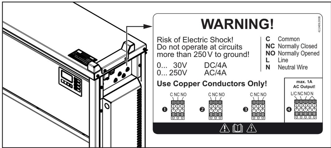
The optional relay board enables the charger's operating statuses and the connected battery's state of charge to be evaluated externally. One or more external consumers can also be supplied with L-N input voltage. A neutral conductor in the electrical mains supply is a prerequisite for this. The configuration of the relay board outputs is explained in the Operating Instructions for the charger: "Additional functions" in the "Display" section.
