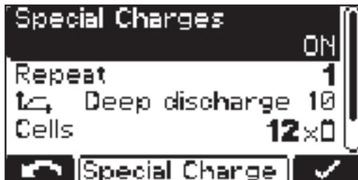
Selecting "Special Charges" allows one or more of the alternative charging types to be performed temporarily.
