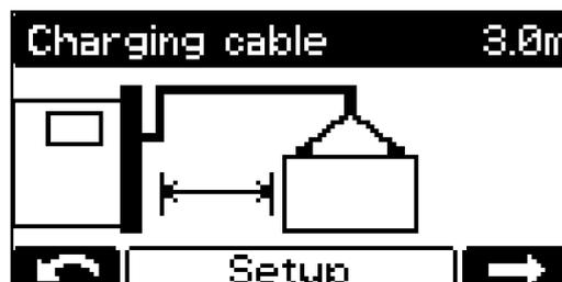
8 Use the "Up/Down" keys to set the length of the charging lead.
