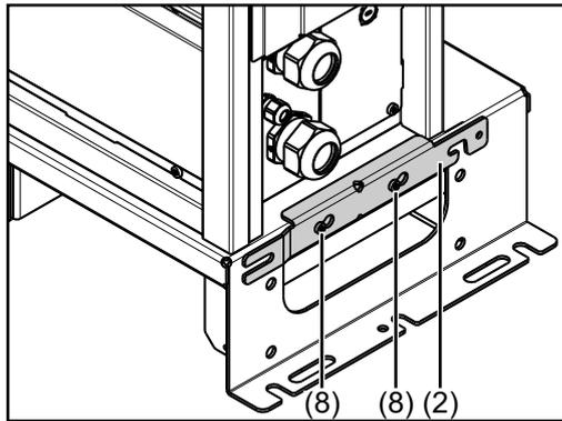
Alternatively, the wall bracket bar (2) can also be stored on the right-hand side of the device. It is secured using TX25 screws (8) and a tightening torque of 3 Nm.
