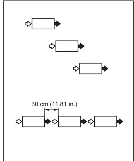
If the chargers are arranged in a line one behind the other without being offset, the minimum clearance between the chargers must be as follows:
