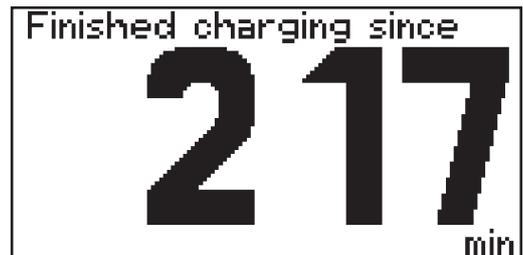
The battery symbol indicates the current state of charge. The greater the number of bars that are displayed, the further advanced the charging process is. As soon as the battery is fully charged, a minute counter will appear (see figure on right). This counts the minutes since the end of charging; when a number of chargers are being used, this makes it easier to decide which battery has already cooled down most.
