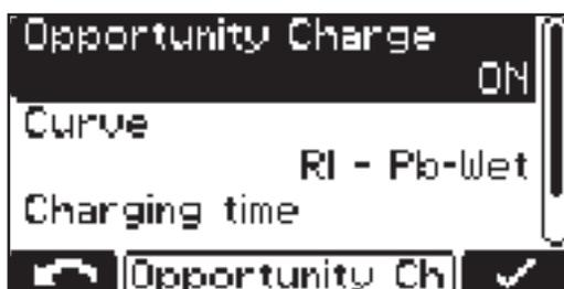
To extend the usage interval of a battery, it is possible to recharge it at a time when it will not be needed, e.g. during scheduled plant shutdowns.
