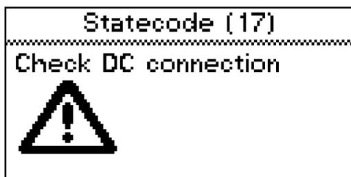
If problems arise with the DC connection during the charging process, status code 17 is set if the DC connection check is active.
