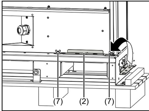
If the wall bracket bar (2) is not required, store it on the rear of device and secure it using wing nuts (7).
