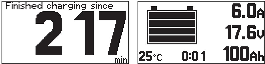
When the battery is fully charged all 4 bars of the battery symbol appear black. As soon as the battery is fully charged, the green indicator lights up.
